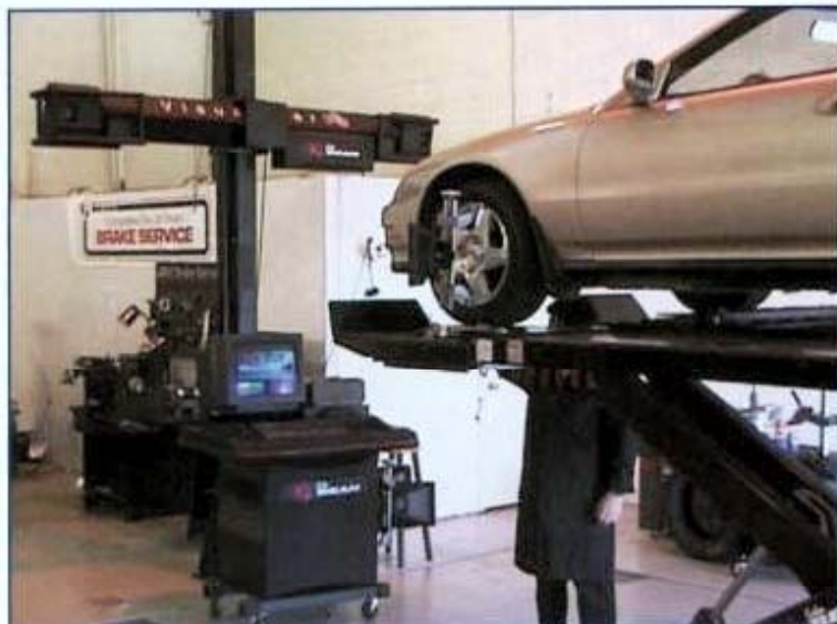
Technician making alignment adjustments using the JBC V3D movable camera boom with the alignment lift in its full up position.
