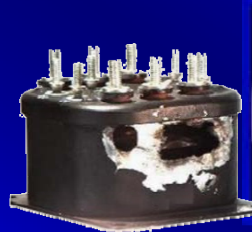
Electromagnetic Relay Short Circuit
